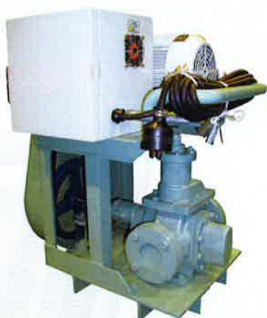
6 Belt drive unit with inverter (change speed)
