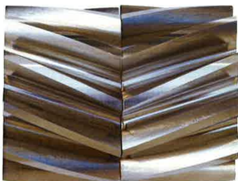
Involute Tooth Profile (Enlarged view)
